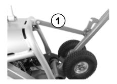
Tilt the machine to the rear and guide it via the guide bar.
