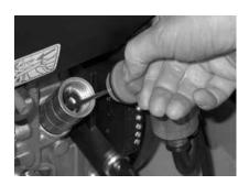
The correct oil level is between the min. and max. marks.
