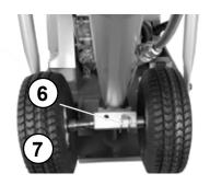
Fasten the wheel (7) on the base plate with the locking pin (6).
