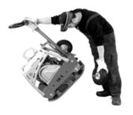
Pull the locking pin (6) out of the holder and remove the wheel (7).
