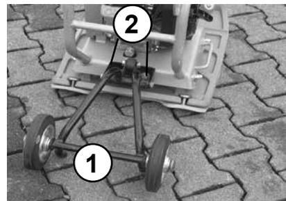
Arrest the guide bar (1) with the spring bolt (2).
