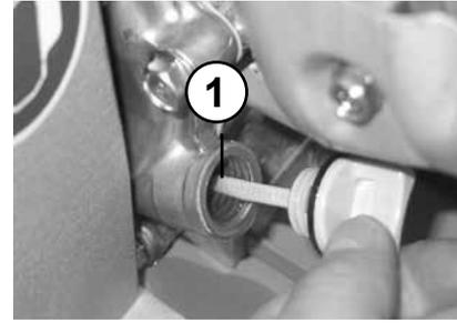
The correct oil level is between the min. and max. marks.
