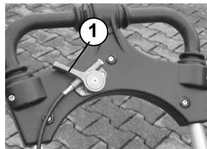
Control drive speed and direction of travel with the handle (2).
