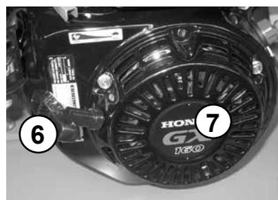
Slowly tighten the handle (6) of the reversing starter (7) until resistance is noticeable.
