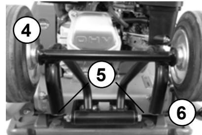
Pivot the undercarriage under the base plate.
